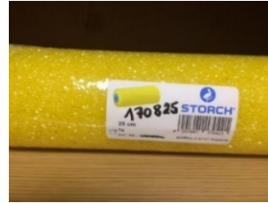
Example of a coarse-pored foam roller - to be used for all the above tackifiers.
